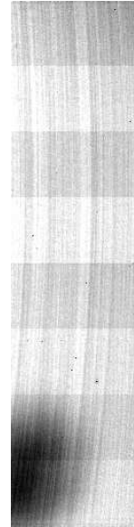
Figure 34: Example of the display aliasing when in subframe modes, here 256 \times 1016 pixels. This is seen primarily when the image is taller than wide ( Nx < Ny ) and the Ny dimension not a power of two.
