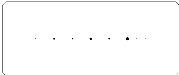
Figure 37: The coronagraphic spot mask. The ten spots project to 0'.1-2'.0 diameter on the sky.
