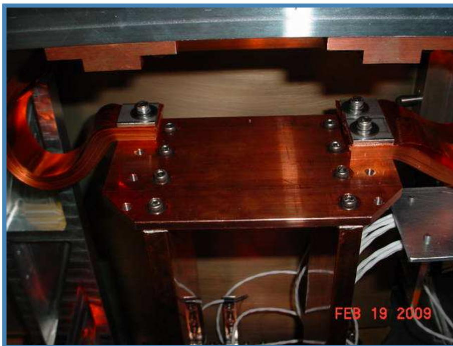
Figure 9. “Cutting corners to improve performance.” The corners that caused a thermal short within OSIRIS have been machined off in this view from the recent servicing mission. They are the two front corners, now at 45 degrees, on the horizontal copper plate at center. Note the cold straps bolted to the back corners of this plate.
