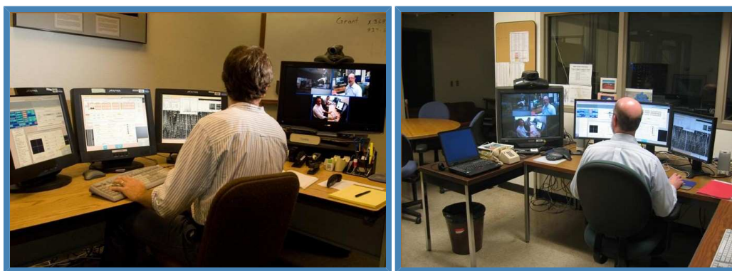
Figure 4. Mainland observing system in operation. Left: Observer in Waimea remote operations room. Right: Observer in Santa Cruz remote operations room. Videoconferencing systems allow audio/visual communication. Similar layouts provide comparable observing experience at all sites. Images courtesy of Sarah Anderson (WMKO) and Steve Allen (UCO/Lick).
