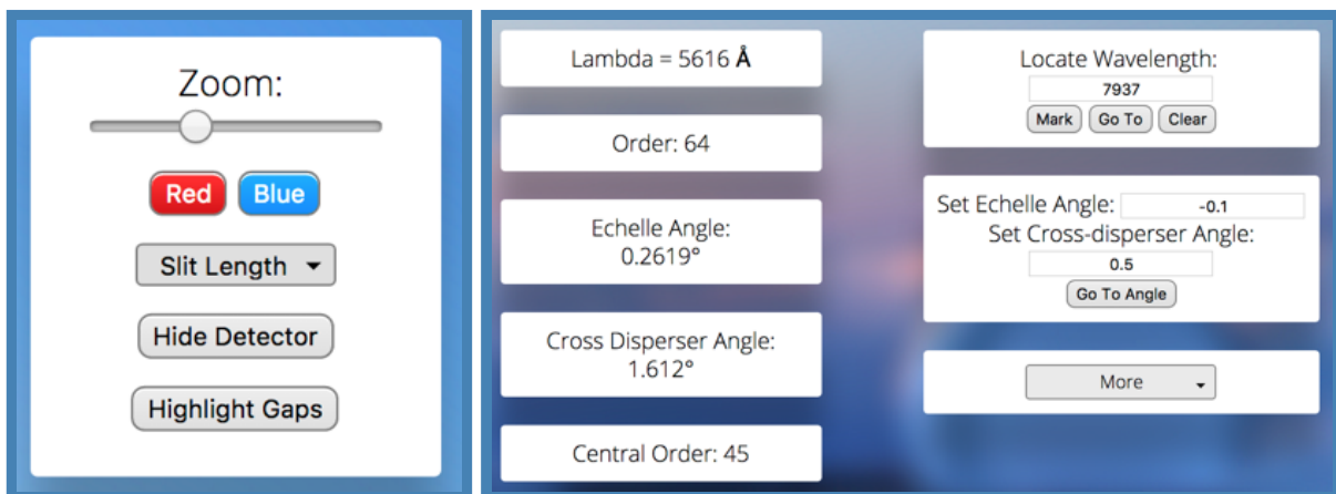
Figure 2. New HIRES EFS control GUIs showing relevant instrument settings for configuring the echelle and cross disperser grating angles and for viewing the resultant wavelength coverage on the detector. *
