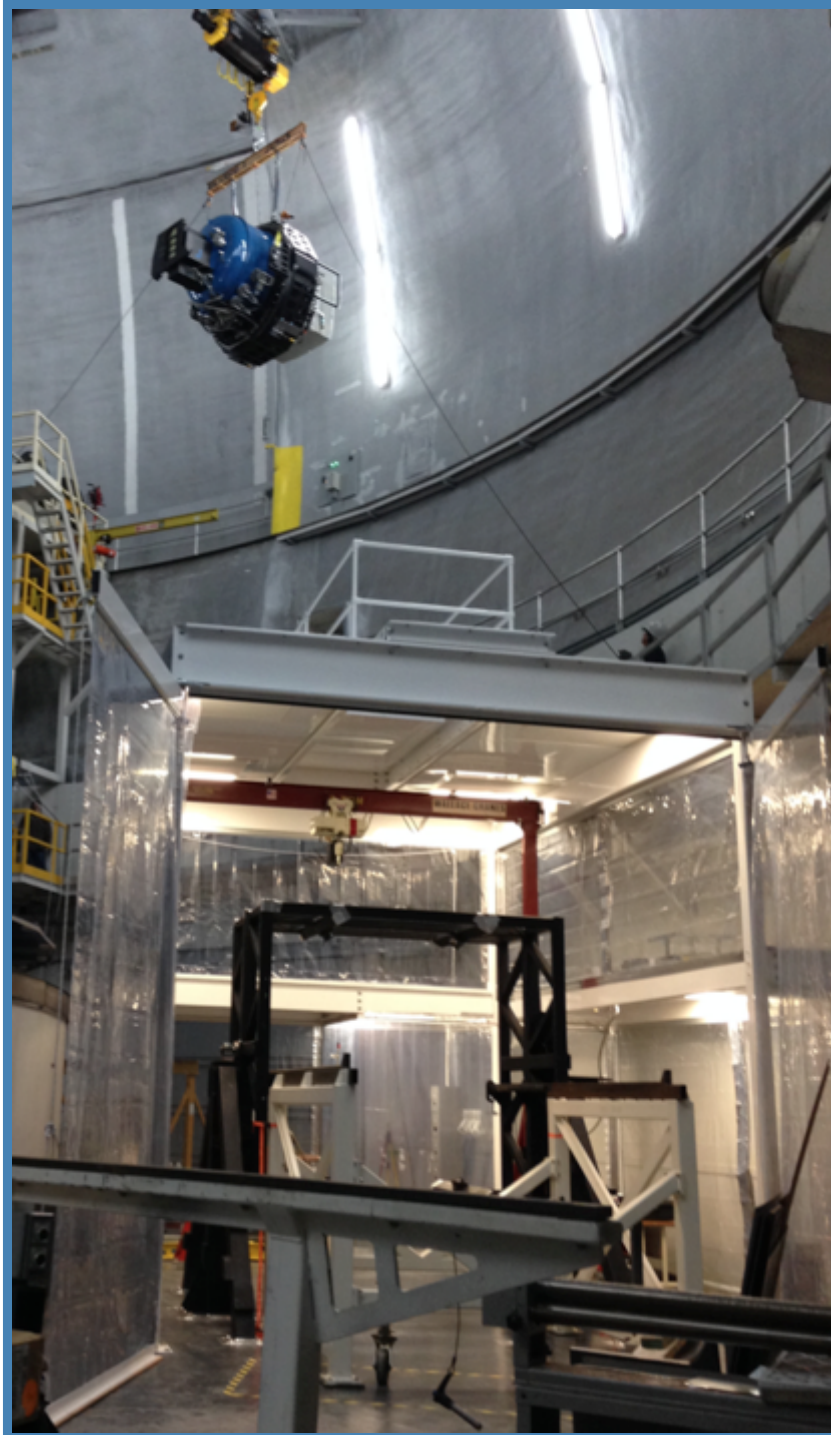
Figure 6. November 3, 2016 MOSFIRE is lifted using the shutter crane from the Keck I deck to the cleanroom on the dome floor. Inside the clean room is the instrument development test stand used to open the instrument. Keck staff completed the clean room in a month.
