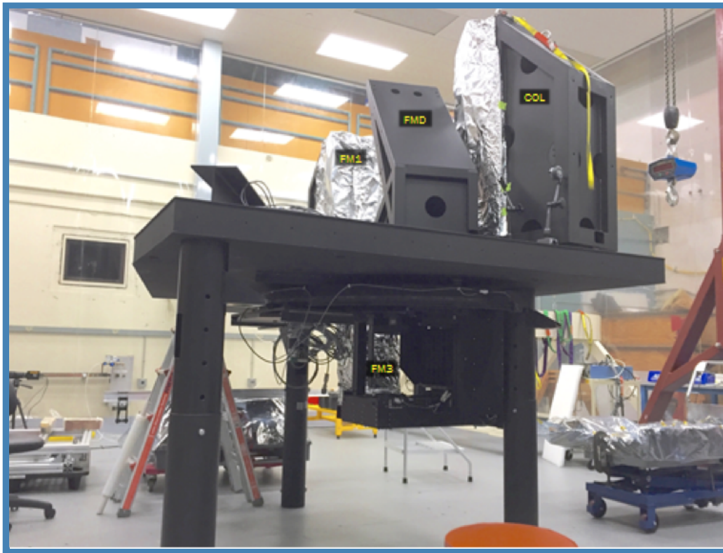
Figure 7. KCWI integration in progress showing the optical bench and the large mirror optics.
