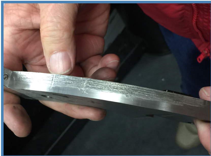
Figure 7. Main driving arc of the tilt mechanism, with scouring marks and deep dents resulting from slippage of the driving gear.
