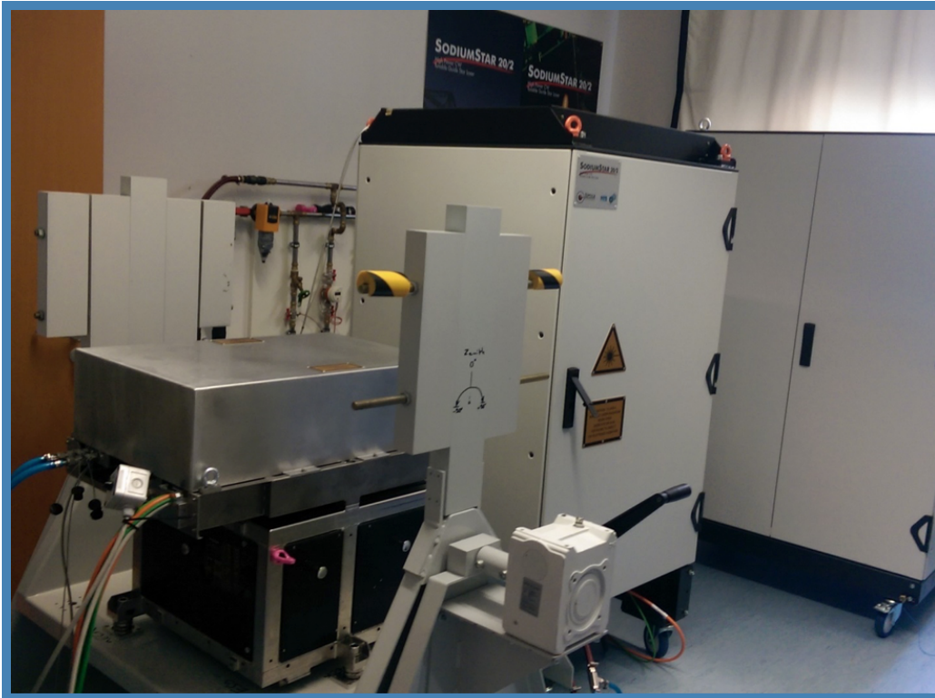
Figure 1. The laser system undergoing gravity testing at the factory. Laser head (left), electronics cabinet (middle), heat exchanger (right).
