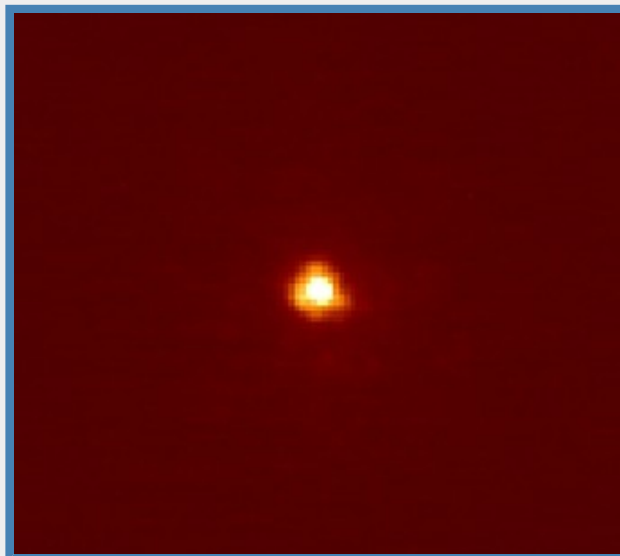
Figure 8. Image of an R \approx 10 mag natural guide star taken with the narrow camera of NIRC2 and the newly installed z filter. The estimated FWHM \approx 30 mas and Strehl ratio \approx 13\% .
