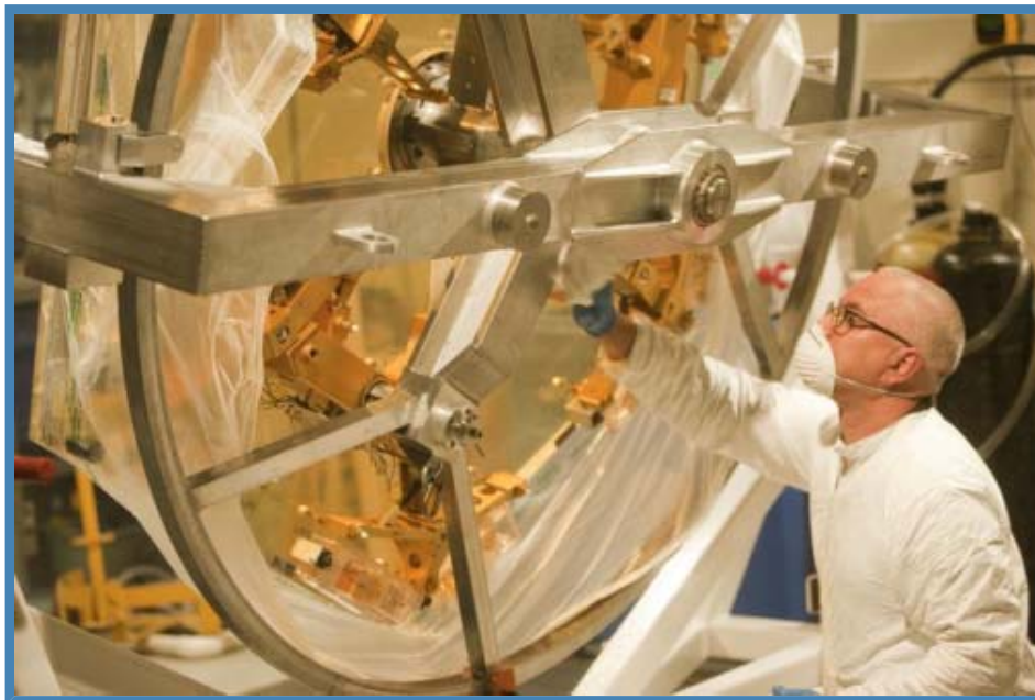
WMKO technician Steve Doyle inspects a primary mirror segment which has been stripped and cleaned in preparation for re-aluminizing.
