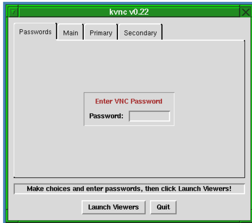
Figure 9. The main screen on kvncgui , our new tool for launching instrument VNC viewers. Simply enter the VNC password and click Launch Viewers!
