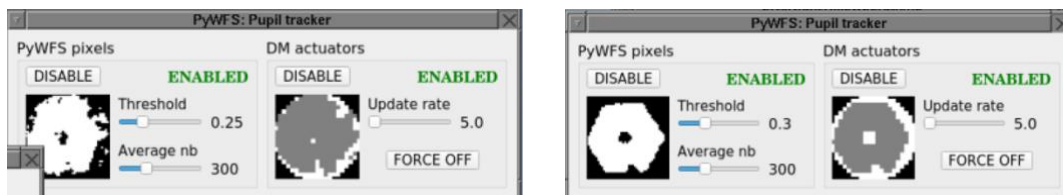
Figure 22: Examples of the PyWFS pupil tracker. Left: Threshold too small leading to too many actuators selected. Right: Threshold adjusted to better select the illuminated actuators.
