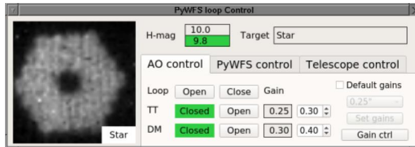
Figure 9: PyWFS loop control GUI, showing the AO control tab. Note: 1 segment missing (seen in pupil illumination map).
