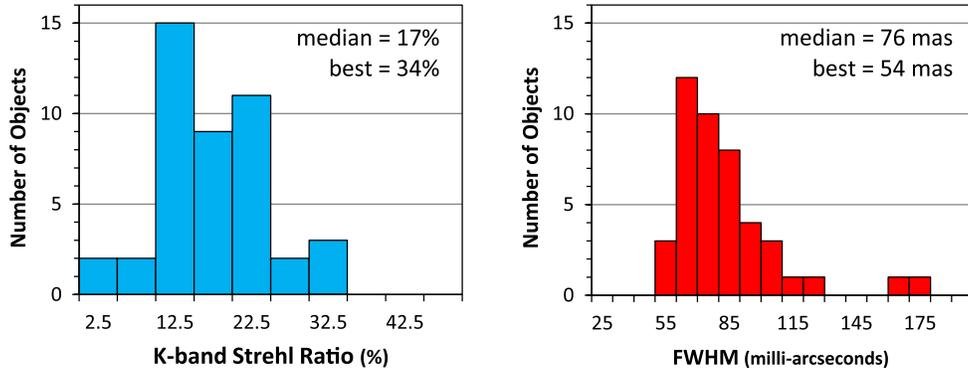
FIG. 10.— $K$ -band Strehl ratio (*left*) and FWHM (*right*) from a Keck II LGS AO survey of field brown dwarfs by Liu (2008). No data was discarded. The data includes a mix of seeing conditions and off-axis tip-tilt star properties. See the electronic edition of the *PASP* for a color version of this figure.
