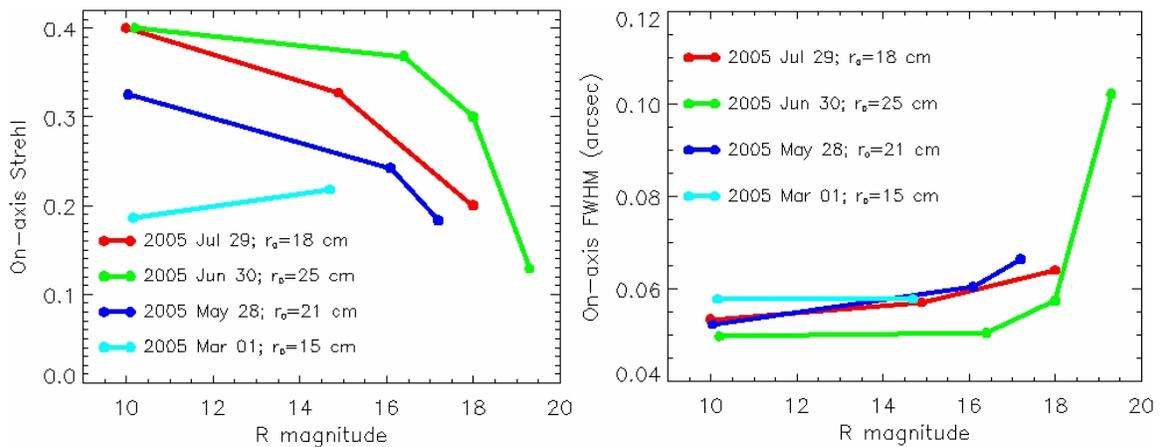
Figure 1: Keck II LGS AO performance measured in 2005. K-band Strehl ratio (left) and FWHM (right) versus seeing conditions and tip-tilt star R-magnitude.
