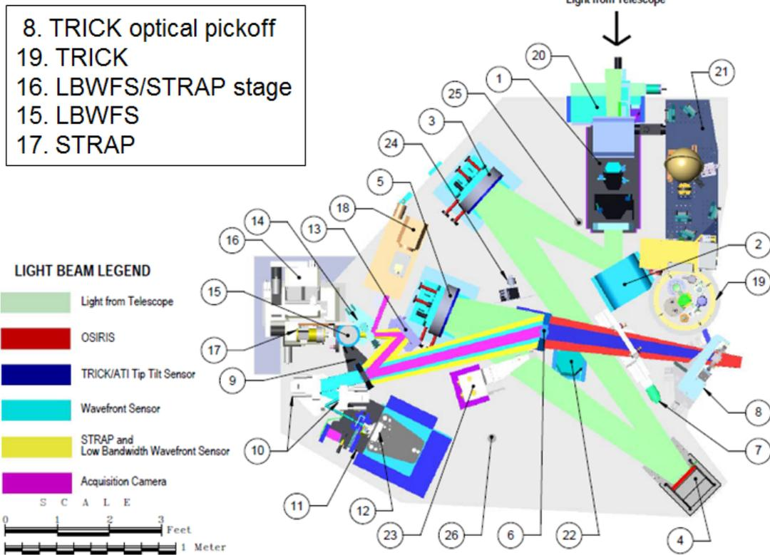
Figure 14: Keck I AO bench with the locations of the STRAP and TRICK hardware. The visible light is reflected by the IR transmissive dichroic at location 6. OSIRIS is located at the AO output at right.
