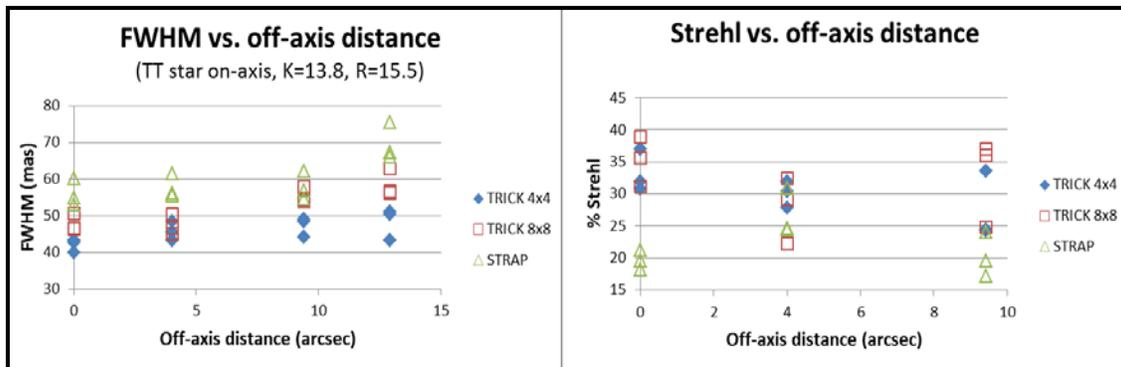
Figure 5: These plots of performance versus off-axis distance show improvement across the OSIRIS imager field with TRICK, indicating the tip-tilt values being measured with this device are more accurate.
