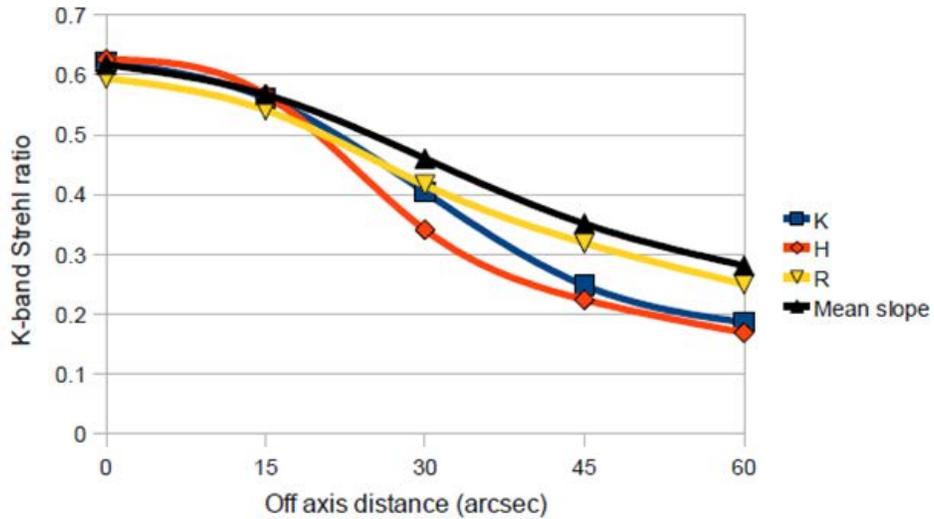
Figure 10: On-axis K-band Strehl degradation as a function of tip-tilt star off-axis distance for a 14<sup>th</sup> magnitude tip-tilt star at three different tip-tilt sensing wavelengths. H and K-band using a 4x4 centroider with 50 mas pixels. R-band using a quad cell with 500 mas pixels.
