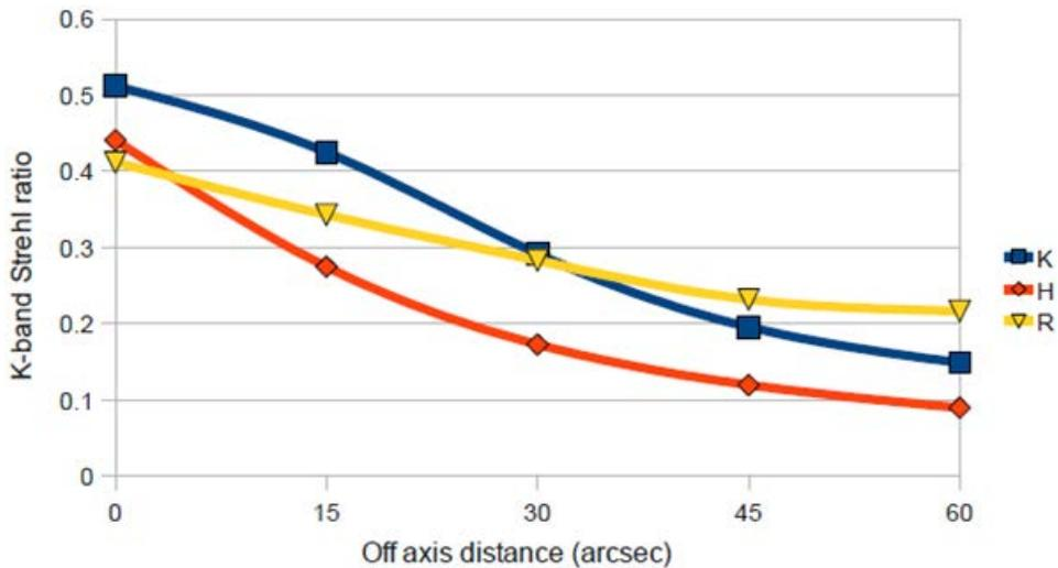
Figure 11: On-axis K-band Strehl as a function of tip-tilt star off-axis distance for a M0 guide star (R=18.5, H=16.5 and K=16). H and K-band using a 4x4 centroider with 50 mas pixels. R-band using a quad cell with 900 mas pixels.
