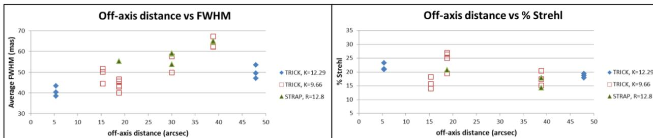
Figure 6: On-axis performance versus tip-tilt star off-axis distance, on the night of August 28, 2015. The Maunakea seeing monitor reported good and stable seeing with a mean of 0.46". The star at 30" was a close binary and was only used for a FWHM measurement.
