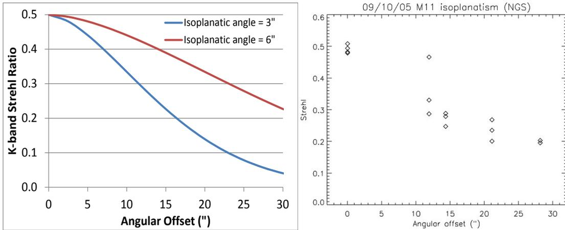
**Figure 8: Left: Predicted K-band Strehl ratio as a function of angular offset from the LGS assuming particular angular offsets. Right: Measured isoplanatic performance from Keck AO data; this plot fits between the two curves in the left plot.**
