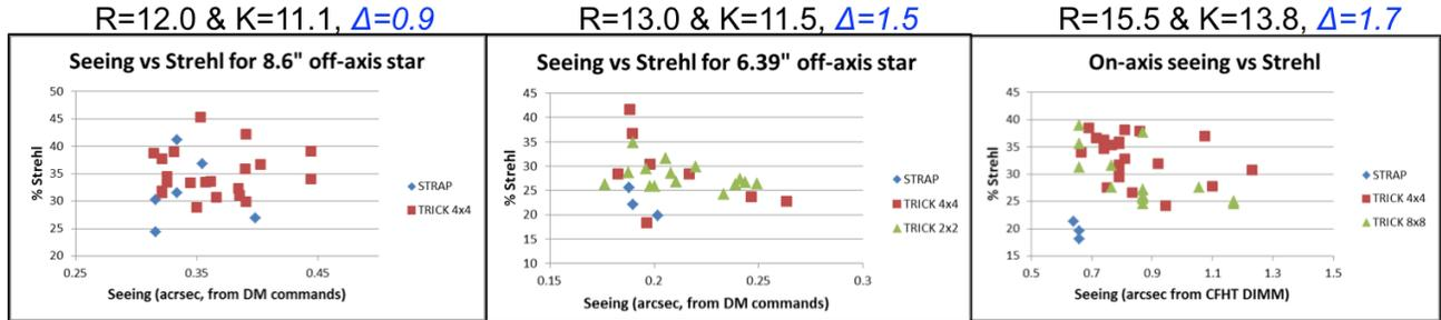
Figure 4: % Strehl ratio with STRAP and TRICK versus seeing for three different on-axis stars. The performance gain when using TRICK is most notable when the difference between the R and K magnitudes is greatest, and when the R magnitude is faintest.
