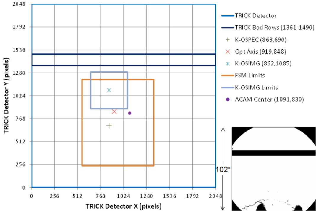
Figure 13: TRICK detector field of regard (102"x102"). The vignettted pixels and bad pixels are shown in the bottom right image. The relative location of the OSIRIS imager and spectrograph are shown.
