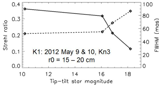
Figure 3: Keck I LGS AO K-band Strehl ratio and FWHM as a function of tip-tilt star R-magnitude (KAON 925).
