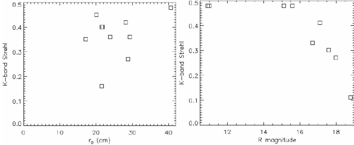
Figure 2: Keck II LGS AO performance measured in 2007 as documented in KAON 489. Left: K-band Strehl versus seeing for a bright tip-tilt star. Right: K-band Strehl versus tip-tilt star magnitude in very good seeing conditions.
