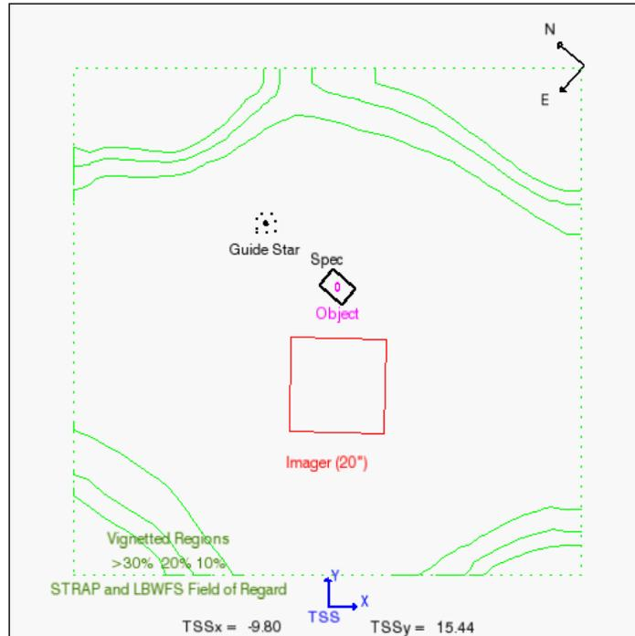
Figure 12: Field of regard within which STRAP/LBWFS can move to acquire a tip-tilt star. A 105"x105" field is shown. The inner most contour line represents 10% vignetting. The relative location of the OSIRIS imager and spectrograph are shown.
