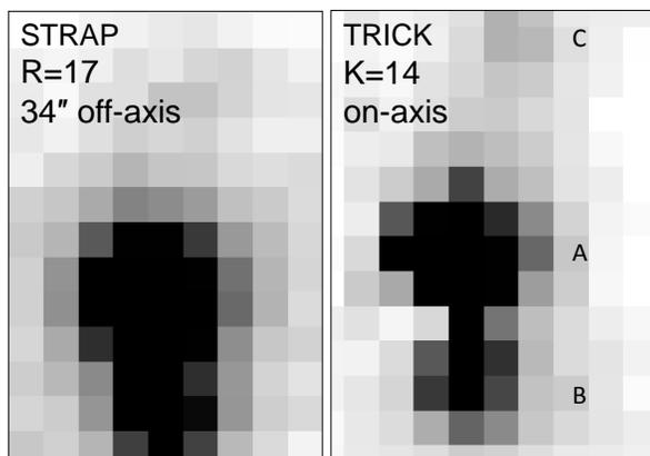
Figure 7: Science performance demonstration. A gravitational lens observed with the OSIRIS spectrograph (25 coadds, 10 minute integration, Hbb filter, 50 mas spaxels). The images are average-collapsed data cubes. A 4x4 pixel region was used on TRICK. The FWHM of an isolated source in the full spectrograph image was reduced from 101x93 mas with STRAP to 76x79 mas with TRICK; and in addition a third source is identified.
