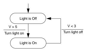
Figure 2-1: A simple state transition diagram
