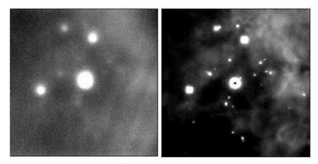
**Figure 1.** First astronomical science from LGS AO, optical (0.65  $\mu$ m) imaging of the central 40" of the Orion Nebula.<sup>10</sup> The image of the left was obtained without AO and the one of the right with LGS AO. This figure was adapted from material on the Starfire Optical Range web site; see Ref. 10 for a higher quality reproduction.
