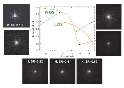
Fig. 9.—(Top) Keck II AO K-band performance versus R-magnitude of the on-axis NGS (as measured by relative counts on the wavefront sensor) under average conditions, as illustrated by a plot of Strehl ratio and NIRC2 images of the NGS. The top-left image is the theoretical perfect point spread function for the Keck telescope. (Bottom) NIRC2 images of the same NGS at J, H and K-band. Adapted from van Dam et al. (2007). See the electronic edition of the PASP for a color version of this figure.
